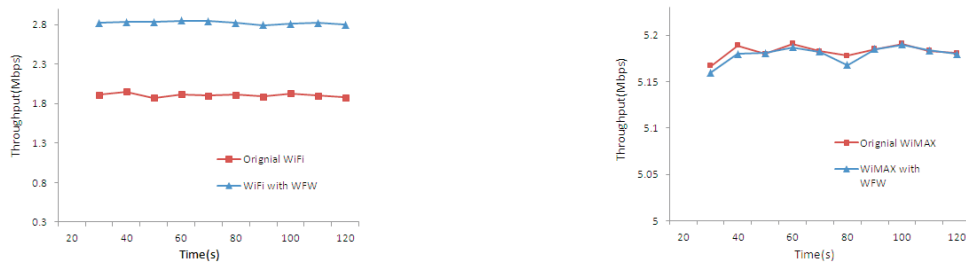
(c) Throughput of WiFi mesh in random distributed scenario (d) Throughput of WiMAX mesh in random distributed scenario
