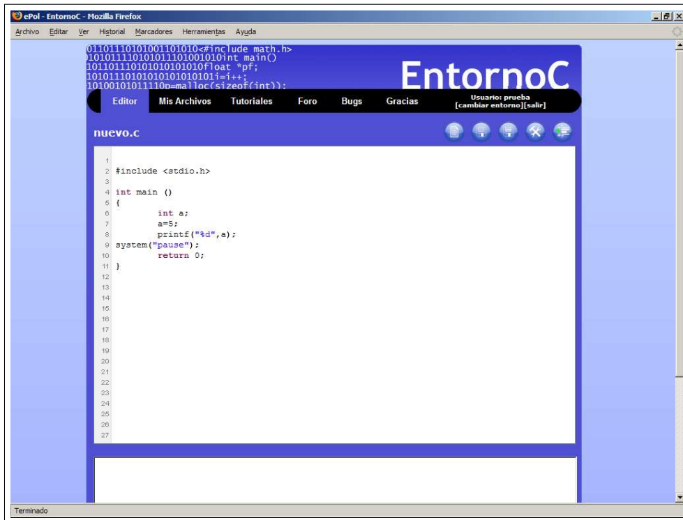
Figure 2: OLC Work screen. With the tabs menu, the tools bar, and two text areas: one for the code and the other one for the results.
