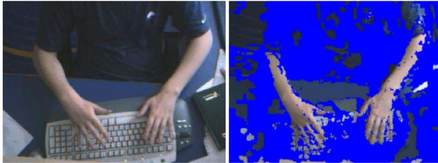
Figure 2: Background subtraction result (blue color indicates the background model)
